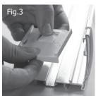
Slide the bracket out of the cassette (Fig.2) and remove the adjustment block (Fig.3). Rotate the adjustment block by up to -1, -2 or -3 **clockwise**.
